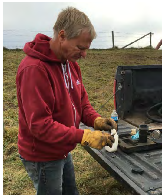
The Agros Nova N meter rapidly estimates the available N content of liquid manure in the field. A chemical reaction is created to evolve ammonia gas which is measured by an attached gauge.
