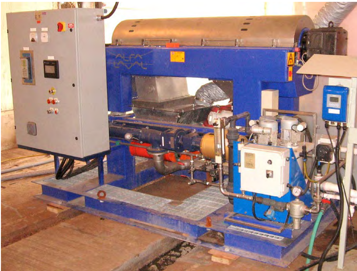
The Alfa Laval centrifuge has a high speed rotating drum that can spin at 4,500 rpm to remove the solids from liquid pig manure.
